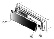
2. Press the left side <sup>©</sup> of the DCP carefully to fit it in place.
